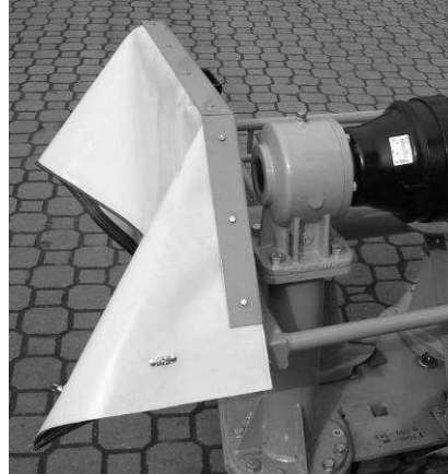
Fig. 10. Mower's side guard lifted for transport
