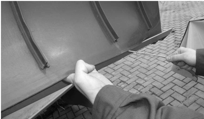
Fig. 36. Removing impurities from inside belt
